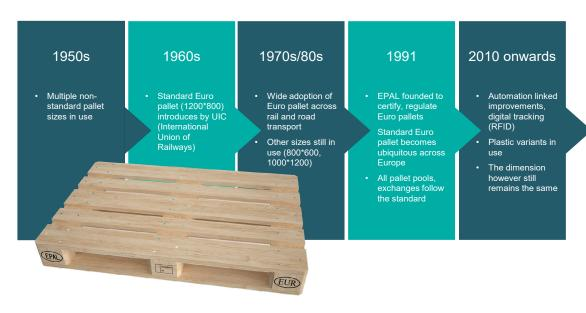
Standardization brings in a lot of efficiencies. The initial euro pallet was developed as a part of an agreement between railways across the countries. It was designed to perfectly fit in European rail cars and trucks, reducing loading time significantly. Following standardization in pallet dimensions, the same has followed in intermodal containers ('pallet wide' containers, with an internal width of 2,440 mm enabling easy loading of 2 pallets side by side).
